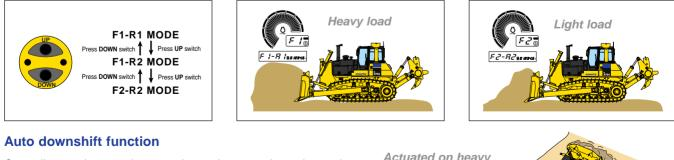
Controller monitors engine speed, travel gear and travel speed. When load is applied and machine travel speed is reduced, the controller automatically downshifts to optimum gear speed to provide high fuel efficiency. This function provides comfortable operation and high productivity without manual downshifting. (This function can be cancelled with cancel switch.) Actuated on heavy load or steep slope
